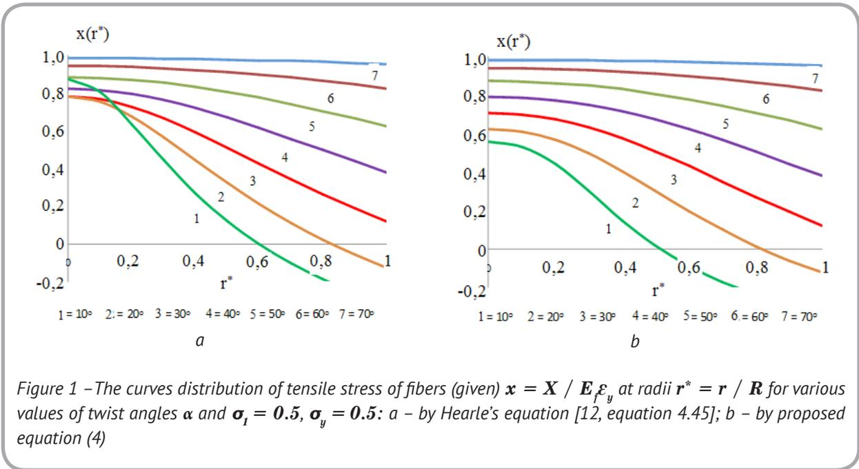
Figure 1 – The curves distribution of tensile stress of fibers (given  $x = X / E_f \varepsilon_y$  at radii  $r^* = r / R$  for various values of twist angles  $\alpha$  and  $\sigma_1 = 0.5$ ,  $\sigma_y = 0.5$ : a – by Hearle's equation [12, equation 4.45]; b – by proposed equation (4)
