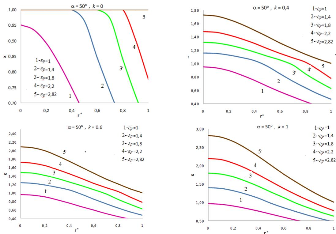
Figure 4 – The curves distribution of tensile stress of fibers (given)  $x = X / E_f \varepsilon_y$  at radii  $r^* = r / R$  at twist angle  $\alpha = 50^\circ$  for various values of  $k = E_{1f} / E_f$  and  $\varepsilon_p = \varepsilon_y / \varepsilon_s$
