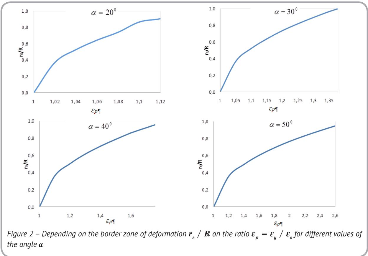
Figure 2 – Depending on the border zone of deformation  $r_s / R$  on the ratio  $\varepsilon_p = \varepsilon_y / \varepsilon_s$  for different values of the angle  $\alpha$
