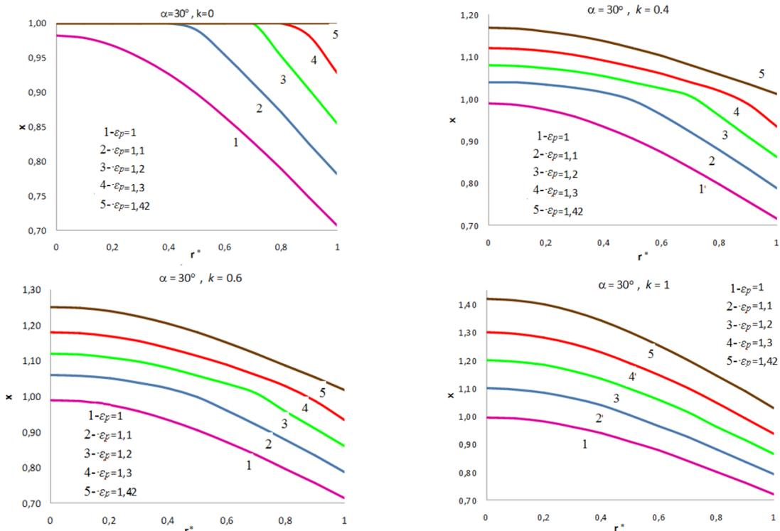
Figure 3 – The curves distribution of tensile stress of fibers (given)  $x = X / E_f \varepsilon_y$  at radii  $r^* = r / R$  at twist angle  $\alpha = 30^\circ$  for various values of  $k = E_{1f} / E_f$  and  $\varepsilon_p = \varepsilon_y / \varepsilon_s$
