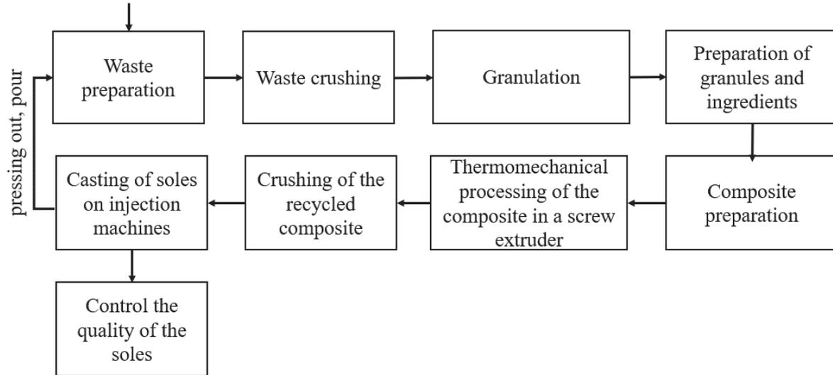
**FIGURE 3.** Technology for producing compositions for the sole of shoes with a fibrous filler
