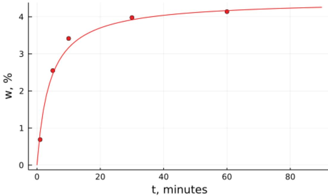
FIGURE 2. Results of hygroscopic properties measurements
