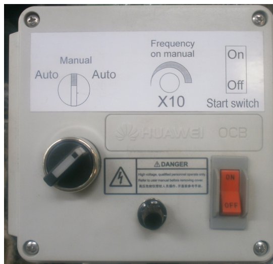
Figure 2 – Remote control of the feed rollers
