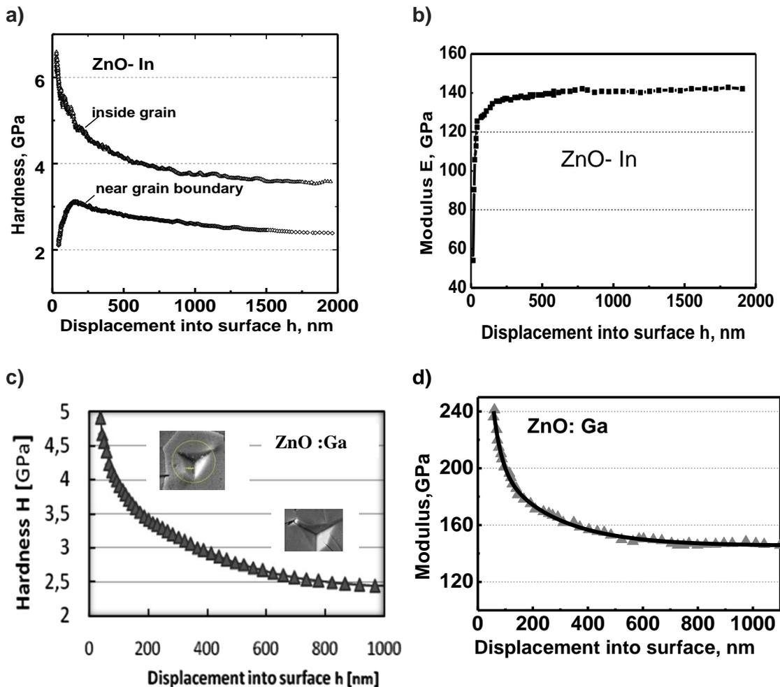
Figure 2 - Hardness H, GPa and Young modulus E, GPa of ZnO-In (a,b) and ZnO-Ga (c,d) ceramics.
