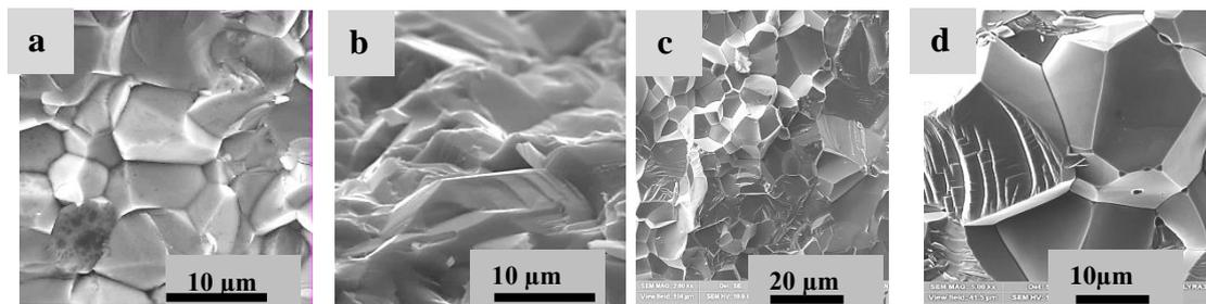
Figure 3 -SEM images of ZnO ceramics fracture: undoped (a), In doped (b) and Ga doped (c,d) ceramics.
