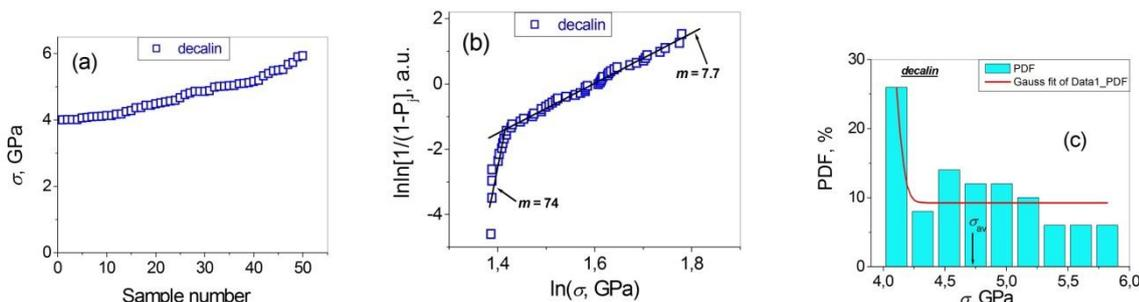
Figure 1 - (a) Tensile strength  $\sigma$  vs sample number shown in ascending order, (b) its Weibull plot, and (c) its Gauss plot (the probability density function, PDF, vs  $\sigma$ ) for the oriented UHMWPE gel-spun single threads
