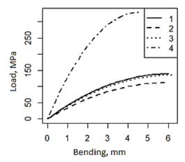
Figure 1 – Deformation of composite materials 1) pure flax fiber preform; 2) 75 % flax fiber, 25 % glass fiber; 3) 50 % flax fiber, 50 % glass fiber; 4) pure glass fiber preform
